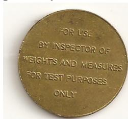
An Inspector's 'test penny' used to operate the coin-in the-slot machines for test purposes
